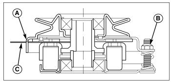
Figure 13. Adjust PTO Clutch
